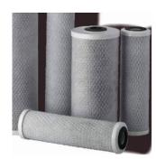
The MOF-E series is formed Acid washed coconut shell activated carbon and is molded together with synthetic fiber binder via a wet production method. Adsorption capacity is unaffected because the surface of activated carbon is not hindered by a binder. So, can maintain high levels of chlorine reduction and chemical adsorptive capacity.
