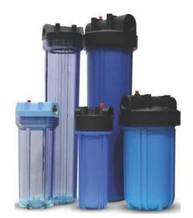
**Opaque Standard Filter Housings** are molded from rugged reinforced polypropylene. They offer outstanding chemical compatibility and are ideal for use in a variety of low-flow applications. These applications include under-sink and countertop residential filtration, pre-and post-reverse osmosis filtration, recreational vehicle filtration, food service and humidifying systems.
