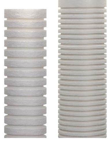
RB (Resin-Bonded) Cartridge is produced from cellulose fibers, which have been intrinsically bonded together by a melamine resin, to create a solid highly durable & porous structure. By treating the fibers in this fashion we can ensure a stronger cartridge that is less likely to collapse than a wound or pleated cartridge.
