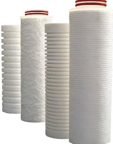
Spun bonded filter cartridges are made up of 100% polypropylene fibers. The fibers have been carefully spun together to form a true gradient density from outer to inner surface. Filter cartridges are available with core & without core version. The superior structure remains integral even under severe operating conditions and there is no media migration. Polypropylene fibers are blown continuously on central molded core, without any binders, resins or lubricants.
